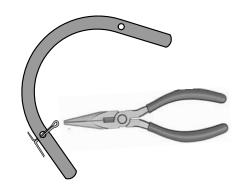
2. SLIDE BAR THROUGH BOTH HOLES LOCATED ON SIDES OF HOUSING.
