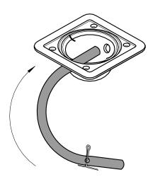
3. SECURE SECOND RETAINING COTTER PIN WITH NEEDLE NOSE PLIERS INTO HOLE ON U-BOLT ANCHORAGE CONNECTOR BAR ON OPPOSITE SIDE OF HOUSING.
