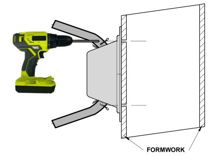
2. SNAP STABILIZER BRIDGE INTO GROOVE LOCATED IN WELL OF THE HOUSING.
