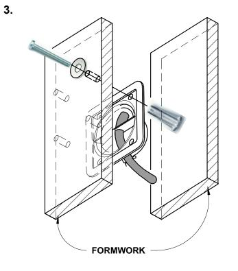
5. PLACE MIN 30 MPa REINFORCED CONCRETE INTO FORM AND VIBRATE CONCRETE.
