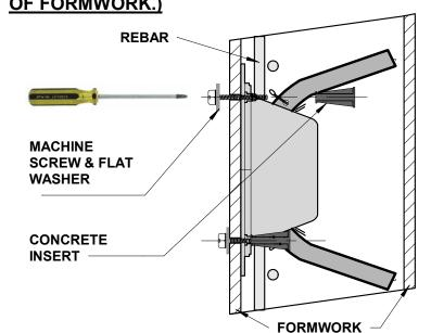
6. REMOVE FORMWORK UPON CURING OF CONCRETE.
